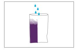
Add sterile de-ionised water as per volume instructions on product (225ml or 3375ml). Add weighed measure of sample material to bag (25g/25ml for 225ml sampling)
